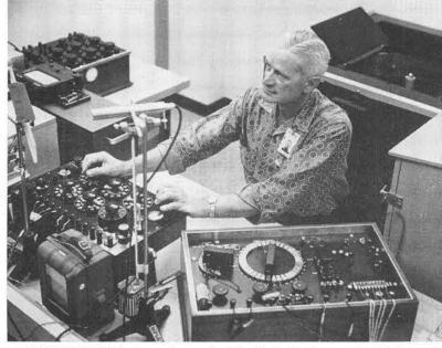
MONITORING temperature of oil bath in background which contains the Primary Lab's standard cells, Neile L. Hensinger (2412-3) prepares to certify standard cells used by secondary labs. The temperature is maintained at 28° within plus or minus .001 of a degree. In the foreground is a standard potentiometer which is used in intercomparing standard cells with primary references.
